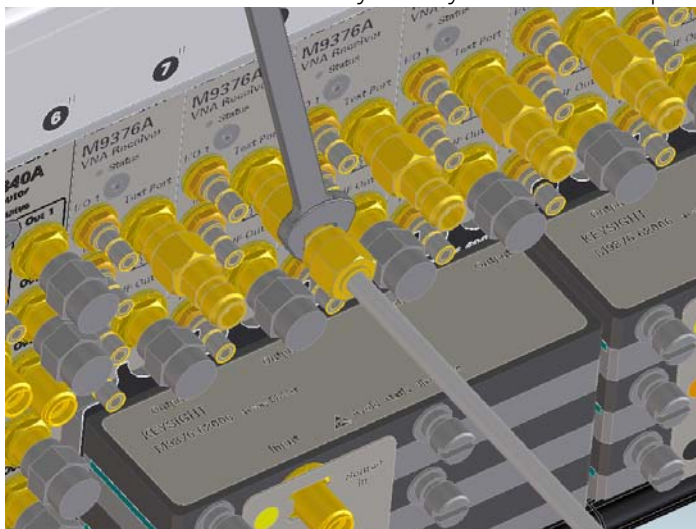
Figure 1-14 Hold the connector saver body steady with 5.5 mm open-end wrench
